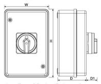
The LVE Metal clad rotary isolator switch range are offered in a number of configuration all rated for installation and use as switch-disconnects and all with options allowing for "lockable off" operation.
